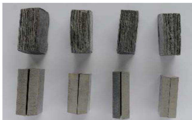
Fig. 2 The first row is lead in the thickness of 12 mm., 12 mm., 10mm and 10 mm. and the second row is tungsten in the thickness of 12mm., 12mm., 10mm and 10 mm. respectively.
